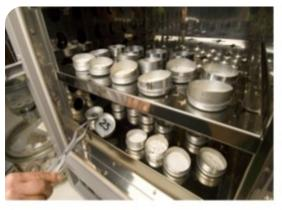
Weight of an empty container with lid =  $W_1$  Weight of container with lid + wet soil =  $W_2$  Weight of container with lid + dry soil =  $W_3$  The calculations are as follows: Weight of dry soil =  $W_3 - W_1$  Weight of water in the soil =  $W_2 - W_3$  Water content,  $w = \frac{\text{Wt of water}}{\text{Wt of dry soil}} \times 100\%$
