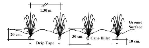
Figure 3. Lay out of plantation and subsurface drip installation
