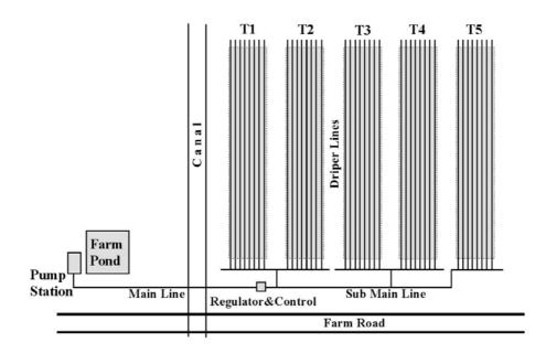
Figure 2. Plan of sugarcane planting plots and drip irrigation system
