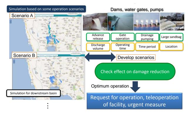
Fig. 10 Simulation for Optimum Operation
