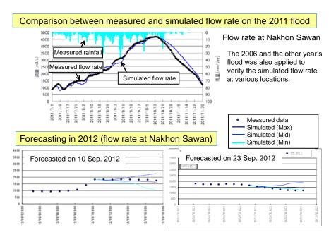
Fig. 3 Forecasting Accuracy (Flow Rate at Nakhon Sawan)
