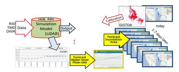
The structure of Flood Risk Information System is schematically shown blow.
