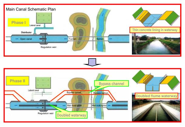
Fig.3 Reconstruction of the main canal
