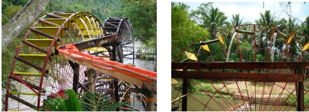
Picture 1. Water intake from lower surface and supply to higher areas by water wheel
