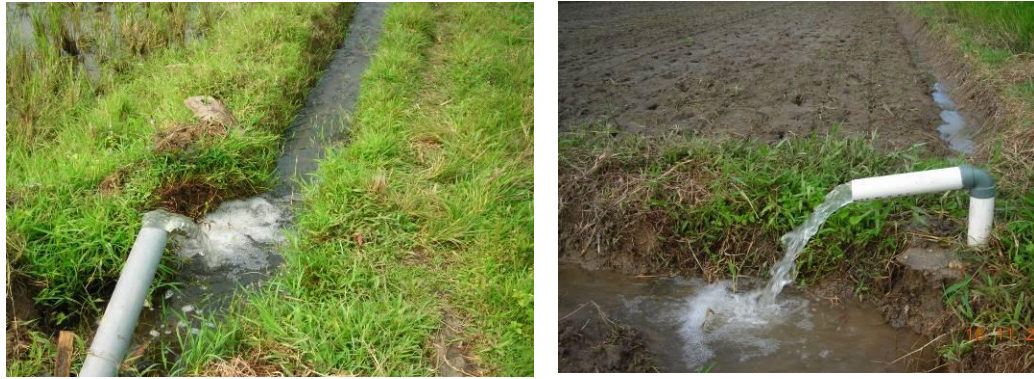
Picture 2 Flow from water wheel directed into irrigation channel (left) and flow from water wheel into paddy field (right)
