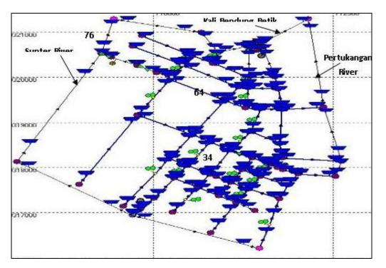
Figure 5. DUFLOW model schematization included the locations of Section 34, Section 64 and Section 76
