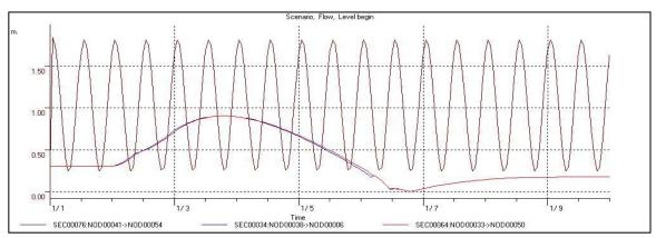
Figure 14. Water levels in Kelapa Gading influenced by land subsidence and sea level rise with the existing pumping capacity
