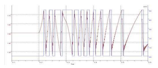
Figure 12. Water levels and pumping discharge at Don Bosco (3) Compartment with the pumping capacity of  $5m^3/s$
